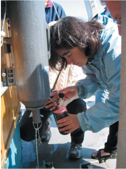
(Left) Informal educator Wendy Wicke collects water from a Niskin bottle aboard the research vessel R/V Gulf Challenger.
